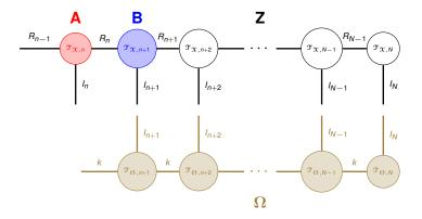
Tensor network diagram: vertices represent tensors, edges represent modes, connected edges represent contractions
