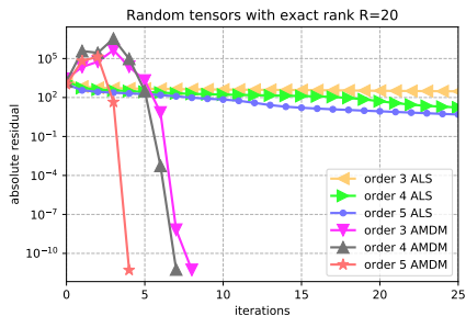
Figure: CP Decomposition of synthetic tensors with rank 20 and 100^3 entries
