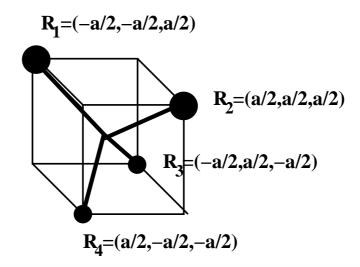
The above figure shows an object with four particles held together with massless bonds at the coordinates shown. The masses of the particles are  $m_1 = m_2 \equiv 2m$  and  $m_3 = m_4 \equiv m$ .
