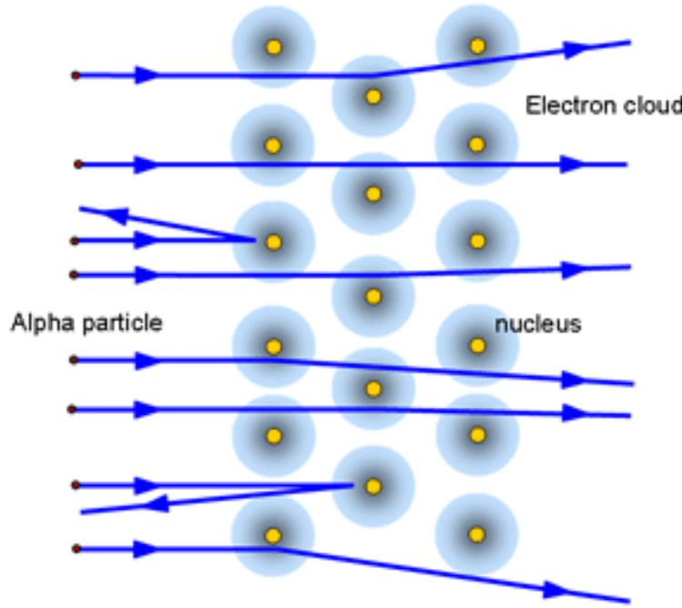
Au target particles consist of Au nuclei which are screened by electrons.
