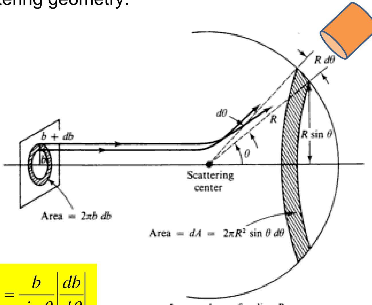
$$\left( \frac{d\sigma}{d\Omega} \right) = \frac{b}{\sin \theta} \left| \frac{db}{d\theta} \right|$$
