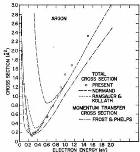
FIG. 2.  $e^-$ -Ar scattering cross sections versus electron energy 0–2 eV.
