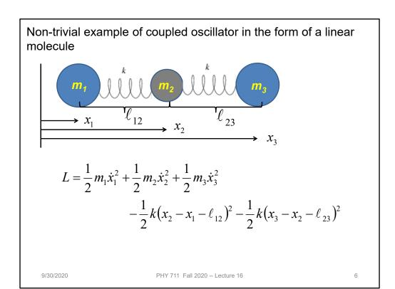
Example with 3 masses connected with springs moving in one dimension
