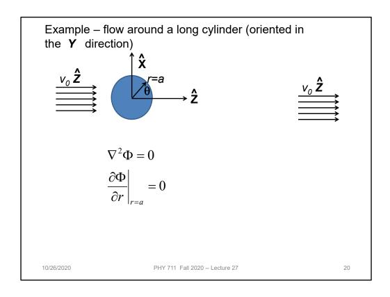
Now consider the uniform fluid in the presence of an impediment. In the is case we consider a cylindrical log.
