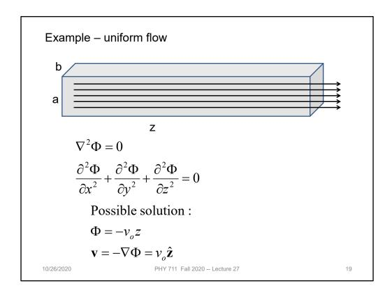
For a uniformly fluid flowing along the z direction, the velocity potential and velocity field are easily written as shown.
