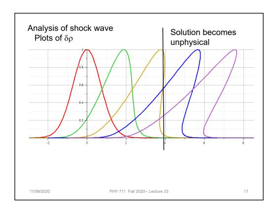
Note that the vertical axis represents the longitudinal wave displacement. When this displacement becomes multivalued for a given coordinate x as shown, the solution becomes unphysical. At this point we need to consider the analysis in a different way.
