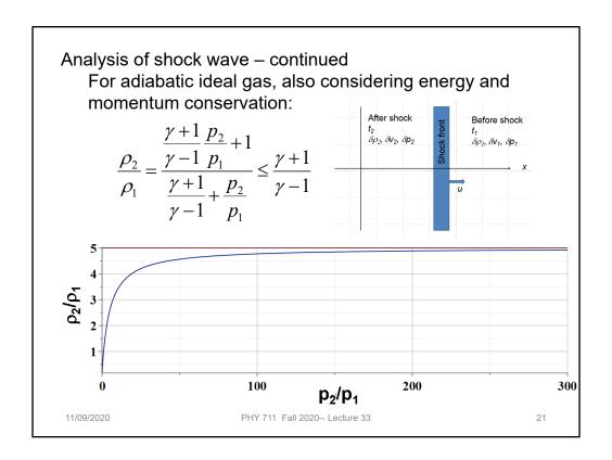
Analyzing ratio of the density after and before the shock wave.
