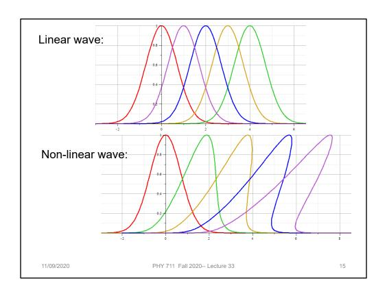
Snap shots of solution for an initial Gaussian waveform for the linear and non-linear solutions.
