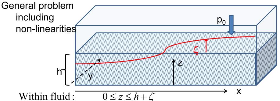
$$-\frac{\partial \Phi}{\partial t} + \frac{1}{2}v^2 + g(z - h) = \text{constant} \quad \text{(We have absorbed)}$$
