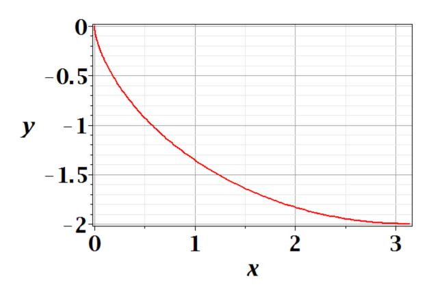
A particle of weight mg travels frictionlessly down a path of shape y(x). What is the shape of the path y(x) that minimizes the travel time from y(0)=0 to  $y(\pi)=-2$ ?
