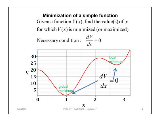
We see from this plot that a conduction for a function to have a minimum at a point is that its derivative is zero at that point. You see in this example another point where dV/dx, but there is not a minimum. So we say the dV/dx is a necessary but not sufficient condition on having a minimum.
