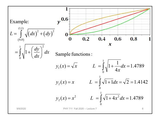
For this example we can write the distance along a curve between two points x=0,y=0 and x=1,y=1 as a normal integral over x as shown.
