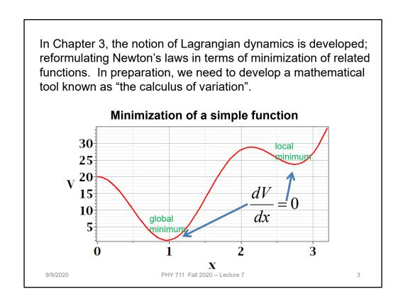
First we should review the notion of a minimum in a continuous function. Here is a plot of V(x) showing two different minima at two different points x.
