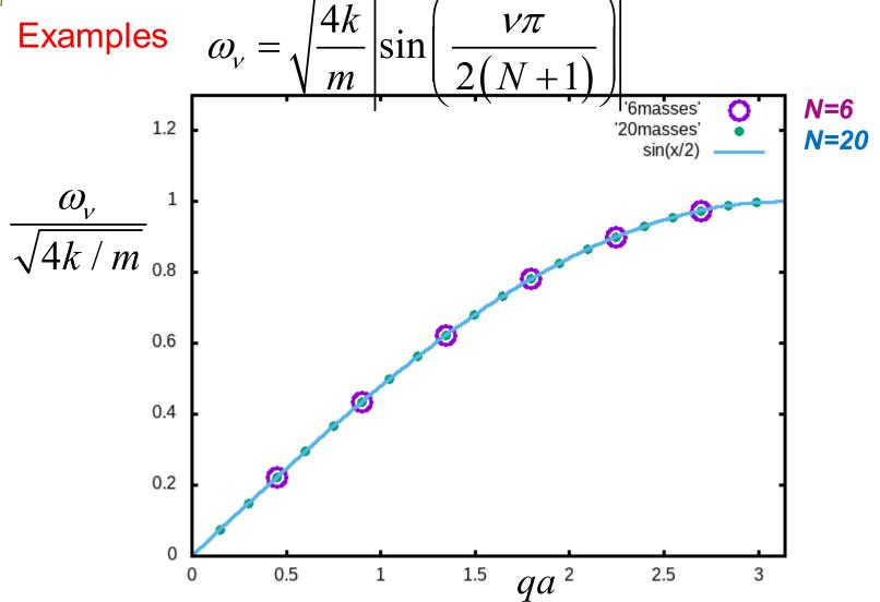
Note that solution form remains correct for  $N \rightarrow \infty$   $\omega(qa) = \sqrt{4k/m} \sin\left(\frac{qa}{2}\right)$
