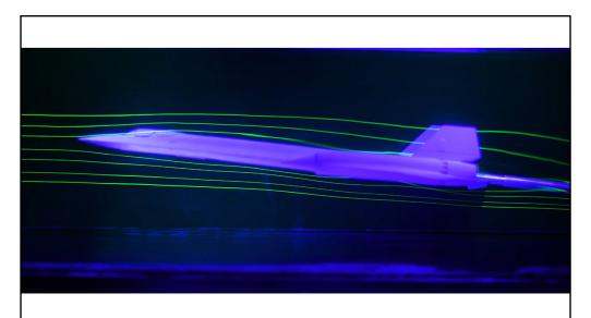
At NASA Ames Fluid Mechanics Laboratory, streamlines of dye in a water channel interact with a model airplane. Credit: *Ian Allen* (copied from Scientific American page mentioned above).
