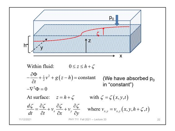
Considering the equations within the wave and at the surface.
