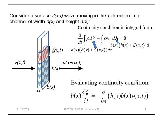
Considering an increment along the propagation direction including the effects of the continuity equation.
