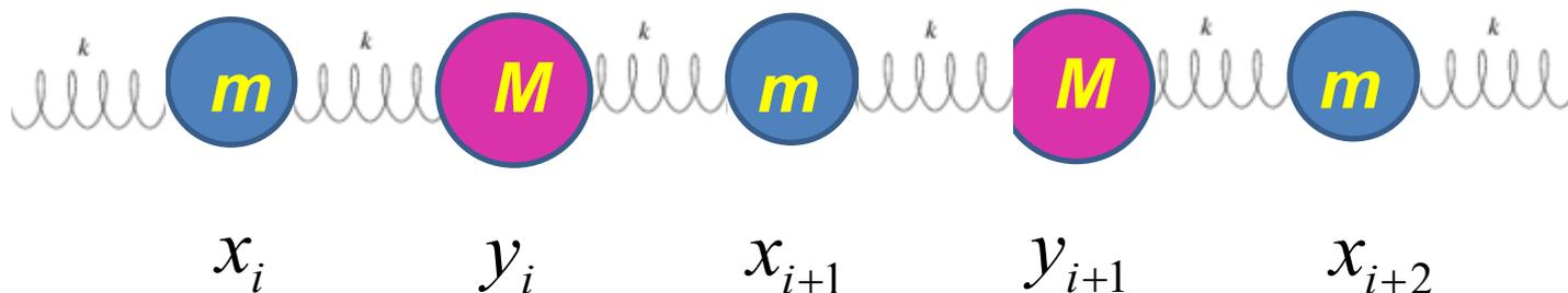
Note: each mass coordinate is measured relative to its equilibrium position  $x_i^0 \equiv 0, y_i^0 \equiv 0, \dots$
