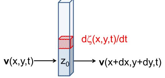
Continuity condition for flow of incompressible fluid:  $\frac{\partial \zeta}{\partial t} + h\nabla \cdot \mathbf{v} = 0$
