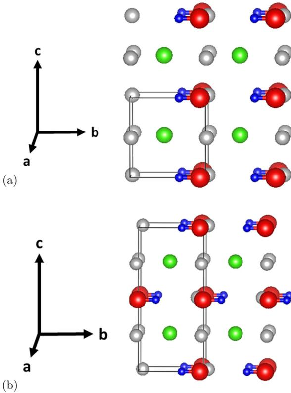
FIG. 1. Ball and stick representations of the computationally optimized structures of  $\text{Li}_2\text{OHCl}$  in the (a) tetragonal structure [space group  $P4mm$  (#99), rotated by  $90^\circ$  about the  $a$  axis from the standard orientation] and (b) orthorhombic structure [space group  $Pmc2_1$  (#26)]. For both structures, green balls represent Cl, red O, blue H, and silver Li.
