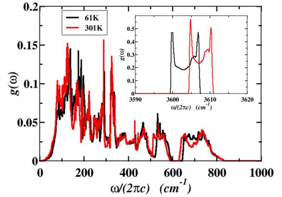
FIG. 2. Plots of  $g(\omega,a,b,c)$  for two different sets of lattice parameters for the orthorhombic phase of  $\text{Li}_2\text{OHCl}$ . The sets of lattice parameters chosen for these plots correspond to optimal parameters found in this work. The inset shows the contributions to  $g(\omega,a,b,c)$  from the high-frequency contributions on an expanded scale, corresponding to the stretching of the OH bonds.
