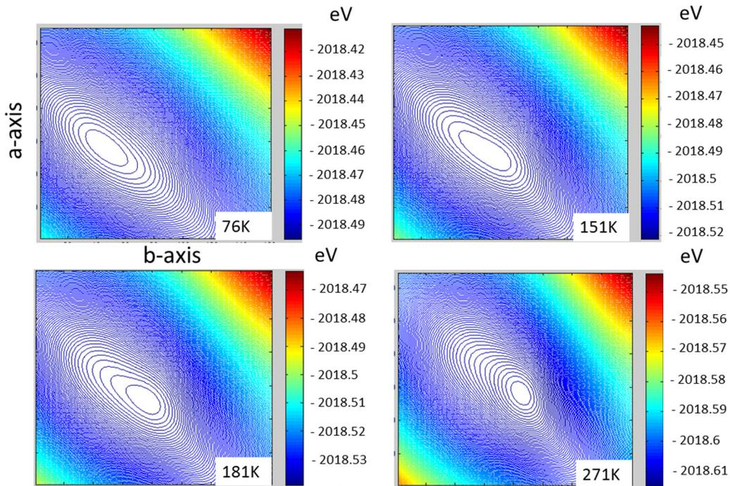
FIG. 7. Contour plots of the computed Helmholtz free energy  $F(T,a,b,c(T))$  of the orthorhombic structure for four representative temperatures  $T$ . For each  $T$ , the plot spans the full grid of points in the  $a$ - $b$  plane at the optimized value of  $c(T)$ . The vertical axis corresponds to the  $a$  axis which spans the range  $3.659 \leq a \leq 3.952$   $\text{\AA}$ , the horizontal to the  $b$  axis which spans the range between  $3.466 \leq b \leq 3.833$   $\text{\AA}$ .
