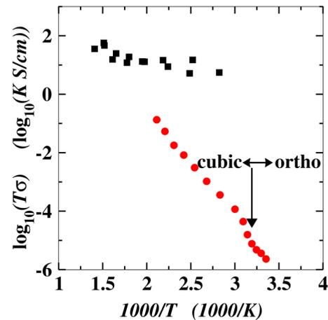
FIG. 11. Red circles correspond to the measured relationship between ionic conductivity  $\sigma$  (S/cm) and temperature  $T$  (in K) for slow-cooled samples of  $\text{Li}_2\text{OHCl}$  plotted as  $\log_{10}(T\sigma)$  versus  $1000/T$ . The black squares correspond to the simulated conductivity inferred from tracer diffusion values according to Eq. (20) in terms of  $\log_{10}(T\sigma H_r)$  versus  $1000/T$ .
