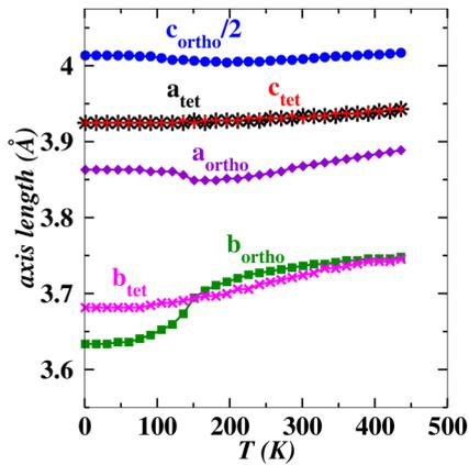
FIG. 4. Comparison of each of the lattice parameters as a function of temperature, calculated by optimizing  $F_{\min}(T)$  at each temperature and by multiplying by 1.02 to account for the systematic LDA error, comparing both the theoretical tetragonal and orthorhombic structures.
