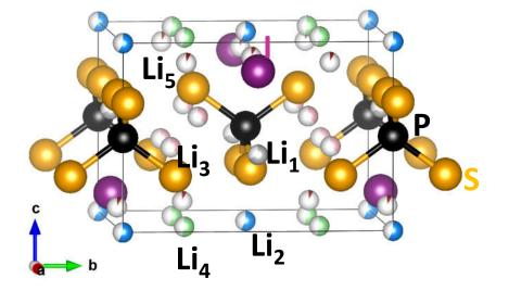
Possible low temperature phase from optimization: *Pmn2*<sub>1</sub> a=8.41 Å, b=8.55 Å, c=6.02 Å 3 fully occupied Li sites
