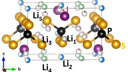
At T=0 K,  $Li_4PS_4I$  is unstable relative to  $\gamma$ -Li<sub>3</sub>PS<sub>4</sub>+LiI.  $Li_4PS_4I \rightarrow \gamma$ -Li<sub>3</sub>PS<sub>4</sub>+LiI+ $\Delta F$
