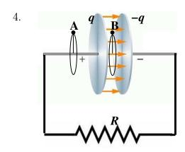
The figure on the left shows a circuit containing a capacitor with  $C=3\times 10^{-8}$  F and a resistance of  $R=2\Omega$ . At time t=0 s, the capacitor is fully charged with  $q(0)=q_0=1\times 10^{-6}$  C. (The capacitor consists of two parallel plates of area A=0.33898 m<sup>2</sup> separated by a distance d=0.0001 m.)
