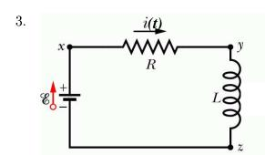
The figure on the left shows a circuit containing a constant emf source  $\mathcal{E} = 5$  V, a resistance of  $R = 5\Omega$ , and an inductor of L = 2 H.
