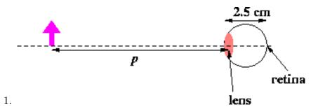
The figure above shows an idealized diagram of a human eye with a variable focus lens located 2.5 cm in front of the retina. The following questions concern the relationships between the object distance p, the focal length of the lens f, and the image distance i, assumed to be on the retina. To receive full credit for this problem, draw at least one appropriate ray diagram and answer questions (a), (b), and *either* (c) or (d).
