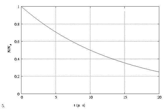
Suppose you have discovered a new unstable particle "A". If you capture  $N_0$  "A" particles in a container (assuming their velocities are essentially zero), the fractional number of undecayed particles present in your container is represented in the plot above, as a function of time ( in  $\mu s$ ).
