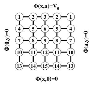
Figure 2:  $5 \times 5$  grid for solution of the Poisson equation within a 2-dimensional square.
