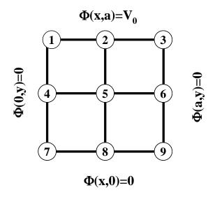
Figure 1:  $3 \times 3$  grid for solution of the Poisson equation within a 2-dimensional square.
