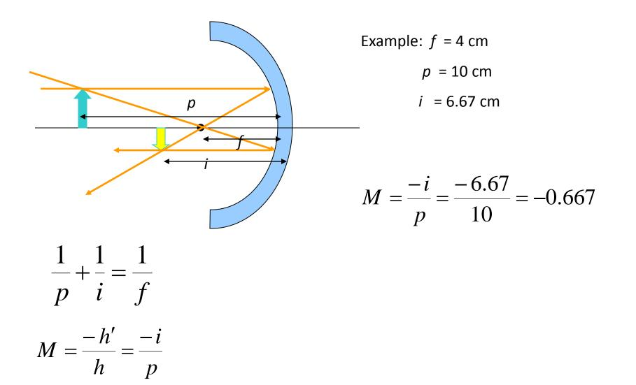
When the object is located so that the center of curvature lies between the object and a concave mirror surface, the image is real, inverted, and reduced in size.
