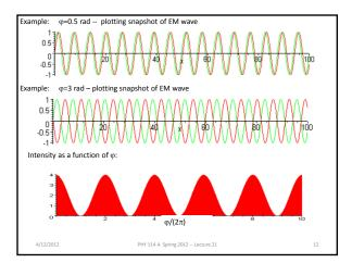
Summary of interference phenomena due to two or more electromagnetic waves which combine at a give point P with path lengths  $r_1$  and  $r_2$  and fixed frequency f.
