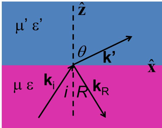
s-polarization –  $\mathbf{E}$  field “polarized” perpendicular to plane of incidence
