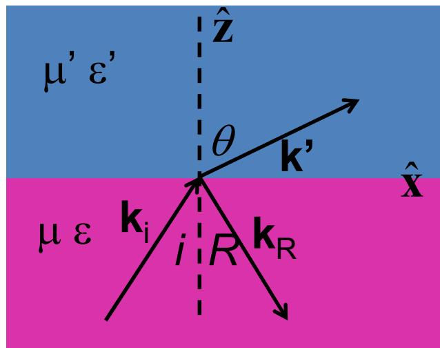
p-polarization –  $\mathbf{E}$  field “polarized” parallel to plane of incidence
