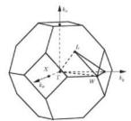
Figure 2.18 Brillouin zone for the face-centered cubic lattice (truncated octahedron). Some high symmetry points are:  $\Gamma=0$ :  $X=(2\pi/a)(1,0,0)$ ;  $L=(2\pi/a)(1/2,1/2,1/2)$ ;  $W=(2\pi/a)(1/2,1,0)$ .
