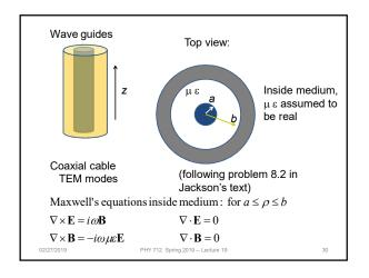
Electromagnetic waves in a coaxial cable -- continued Top view: Example solution for  $a \le \rho \le b$
