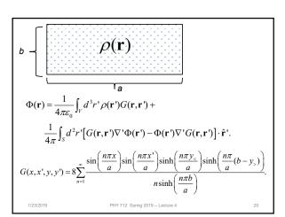
$$G(x,x',y,y') = 8 \sum_{n=1}^{\infty} \frac{\sin\left(\frac{n\pi x}{a}\right) \sin\left(\frac{n\pi x'}{a}\right) \sinh\left(\frac{n\pi y_{s}}{a}\right) \sinh\left(\frac{n\pi}{a}(b-y_{s})\right)}{n \sinh\left(\frac{n\pi b}{a}\right)}.$$
