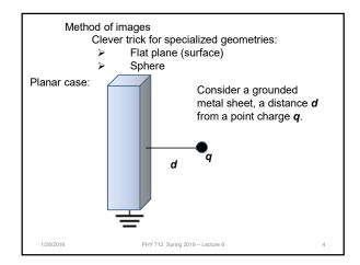
A grounded metal sheet, a distance d from a point charge q. Mobile charges from the "ground" respond to the force from the charge **q**. 1/28/2019 PHY 712 Spring 2019 - Lecture 6
