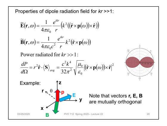
Geometric properties of dipolar fields.
