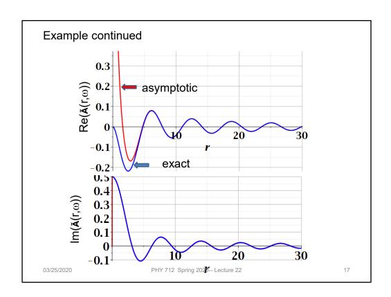
Comparing the values of the vector potential calculated using the asymptotic expansion  $(r\rightarrow infinity)$  with the exact evaluation. You see that the difference occurs only within the source extent.
