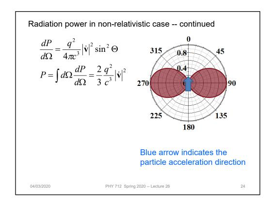
Here we illustrate the non-relativistic power distribution, showing that the radiation intensity is concentrated in the directions perpendicular to the particle acceleration. Next time we will see how relativistic effects change this radiation pattern.
