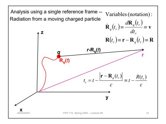
Here we consider a charged particle (charge q) moving along the red trajectory. The vector  $\mathbf{r}$  indicates the point at which we will evaluate the fields. The retarded time  $t_r$  is defined here.
