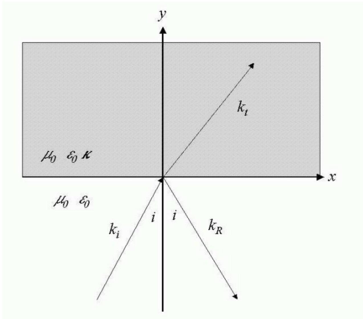
Consider the problem of determining the reflectance from an anisotropic medium with isotropic permeability  $\mu_0$  and anisotropic permittivity  $\varepsilon_0 \boldsymbol{\kappa}$  where:
