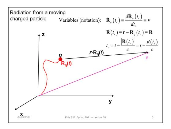
Here is the general diagram we have been using to denote the field point r and the trajectory  $R_q(t)$ .
