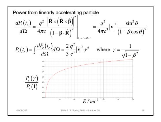
Integrating over solid angle, we obtain the total retarded time power radiated, finding it to vary as gamma<sup>6</sup>. The logarithmic plot shows the gamma dependence.
