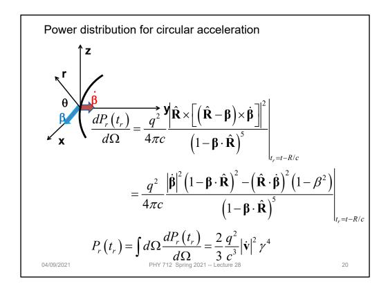
Now consider the case where the acceleration is perpendicular to the instantaneous velocity as in the case of circular motion. In this case, the retarded time power depends on gamma<sup>4</sup>. Check whether you agree with this result (or not). Note that in this diagram the polar angle is not the conventional one.
