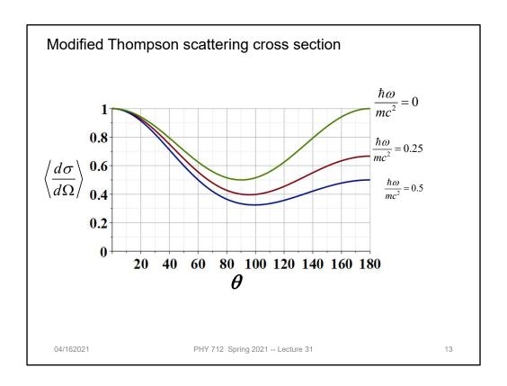
Plot of the changes to the Thompson cross section due to the Compton effect.
