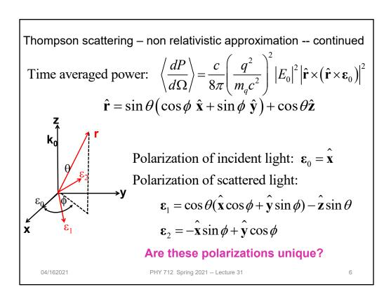
By evaluating the radiation geometry, we can determine the power distribution.
