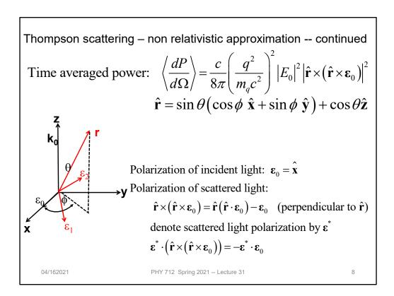
The radiated field is polarized perpendicularly to the propagation direction so that the power depends on the dot product of radiation polarization and the incident polarization.
