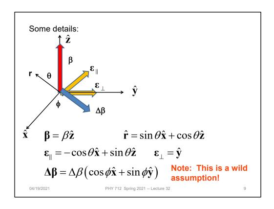
Showing the detailed geometry of the scattering process.
