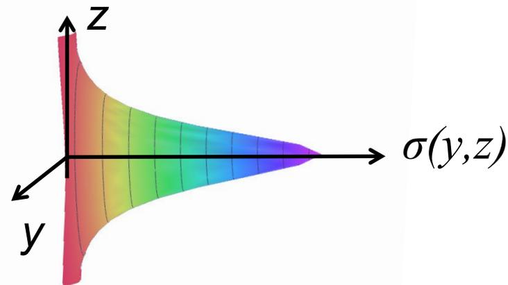
A grounded metal sheet, a distance  $d$  from a point charge  $q$ .
