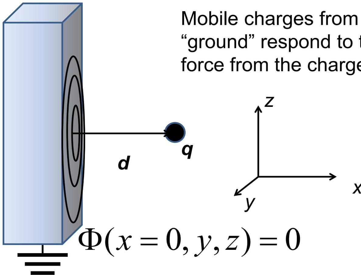
A grounded metal sheet, a distance  $d$  from a point charge  $q$ .
