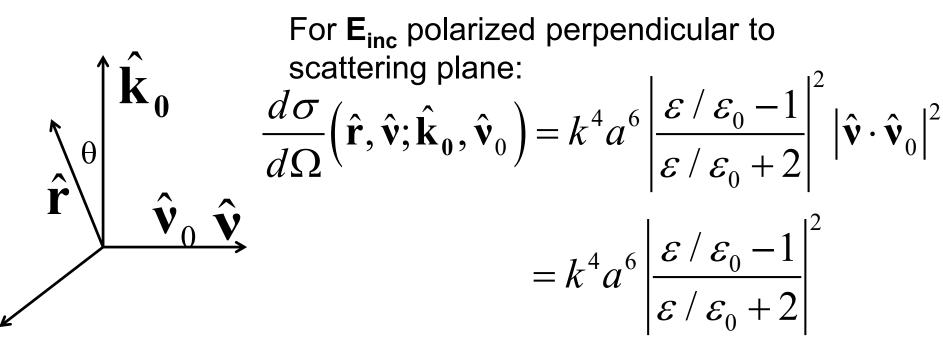
Assuming both incident polarizations are equally likely, average cross section is given by:
