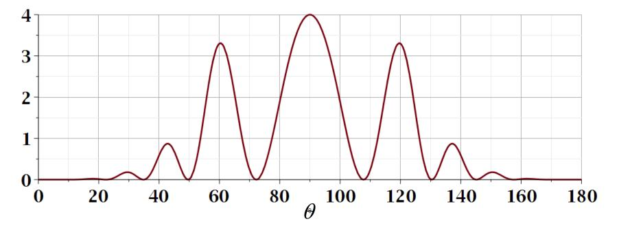
Additional amplitude patterns can be obtained by controlling relative phases of antennas.
