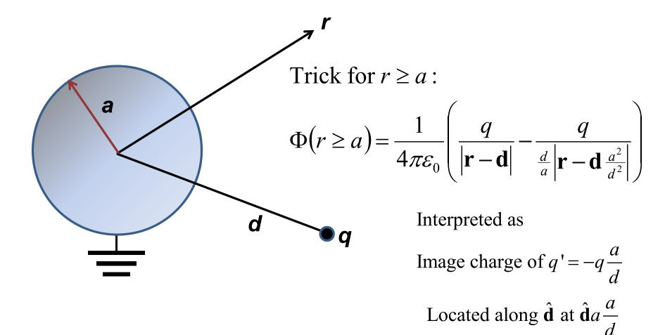
A grounded metal sphere of radius a, in the presence of a point charge q at a distance d from its center.
