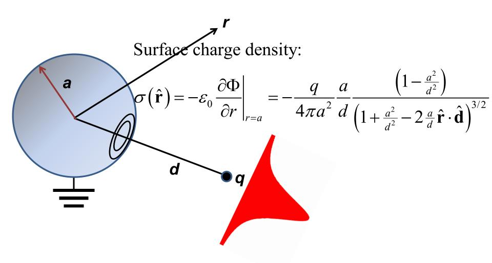
A grounded metal sphere of radius a, in the presence of a point charge q at a distance d from its center.
