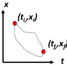
$$S(i,f) = \int_{t_i}^{t_f} L(x,\dot{x},t)dt \qquad L(x,\dot{x},t) = \frac{1}{2}m\dot{x}^2 - V(x)$$
