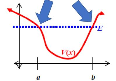
**Figure 12-3:** A potential well that smoothly crosses the energy line at the two classical turning points a and b.
