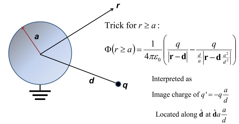
A grounded metal sphere of radius a, in the presence of a point charge q at a distance d from its center.
