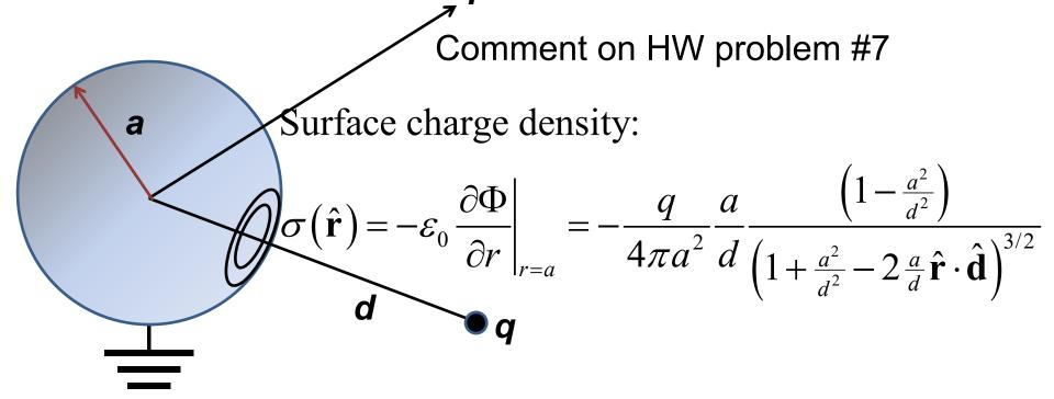
For #1, integrate the charge induced on the outer surface of the sphere due to the point charge q at the point d > a.
