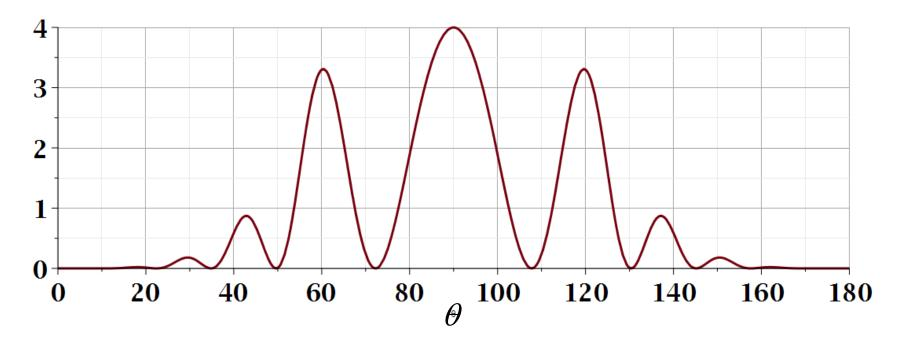
Additional amplitude patterns can be obtained by controlling relative phases of antennas.
