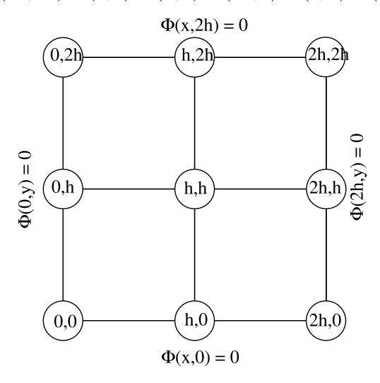
$3 \times 3$  grid for solution of the Poisson equation within a 2-dimensional square.
