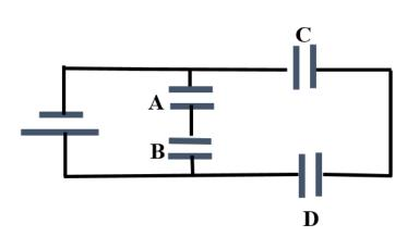
capacitances of the capacitors are as follows:  $C_A = 2$  F,  $C_B = 4$  F,  $C_C = 3$  F and  $C_D = 6$  F (a) Find the equivalent capacitance of the entire assembly. Determine the (b) charge on and (c) voltage across each of the four individual capacitors.
