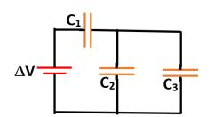
potential of  $\Delta V = 12 \text{ V}$ ,  $C_1 = 3 \mu\text{F}$ ,  $C_2 = 2 \mu\text{F}$ , and  $C_3 = 4 \mu\text{F}$ . (a) Find the equivalent (total) capacitance of the circuit and (b) the charge on and (c) voltage across each capacitor. Enter your answers for parts b and c in the Table below.
