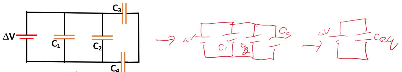
$$C_s = \left( \frac{1}{3} + \frac{1}{6} \right)^{-1} = 2 \mu F \quad C_{eq} = 5 + 2 + 2 = 9 \mu F, \quad Q_{eq} = C_{eq}V = 9 \cdot 9 = 81 \mu C$$
