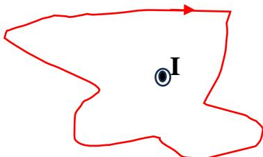
$$\begin{aligned} \oint \vec{B} \cdot d\vec{s} &= \mu_0 I_{\text{enc}} \\ &= (4\pi \times 10^{-7})(2) = 8\pi \times 10^{-7} \text{ T-m} \\ &= 2.5 \times 10^{-6} \quad (\text{T-m} = \text{N/A}) \end{aligned}$$
