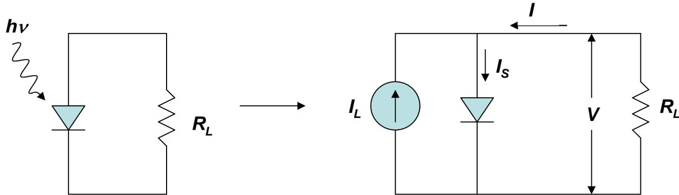
Since the solar cell is essentially a diode, it has the I-V characteristics of one
