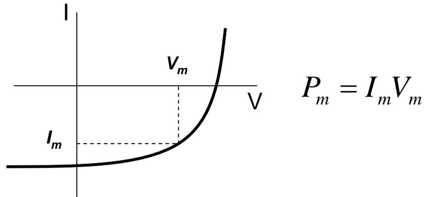
Overall solar cell efficiency:  $\eta = \frac{P_m}{EA_c}$
