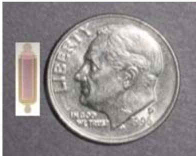
Miniature thin film lithium battery on a ceramic substrate for use in an implantable medical device.
